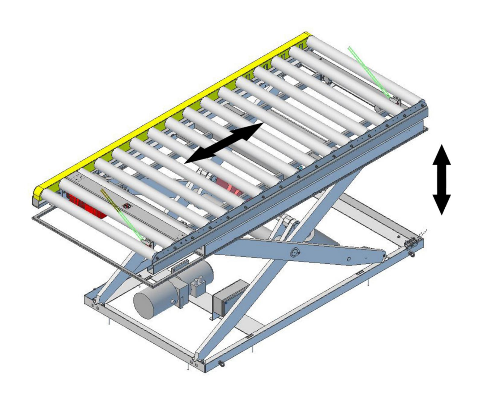
Hydraulic lifting tables are hydraulically driven devices equipped with roll conveyors of different types for the transportation of wood board packets. Integrated hydraulic lifting tables enable the levelling of planes in both mechanical production and manual operation. They are used in co-operation with storing and sorting devices. They may work independently as independent machines or can be furnished in transporting systems.
